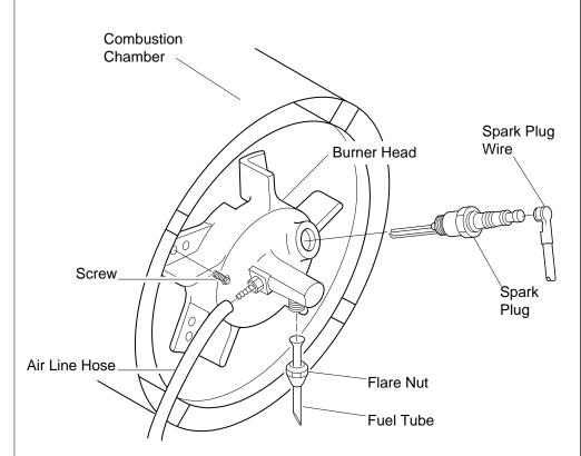
Figure 16 - Removing Burner Head, 150,000 BTU/Hr Model
